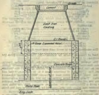
Fig. 7.—Concrete Vault.
